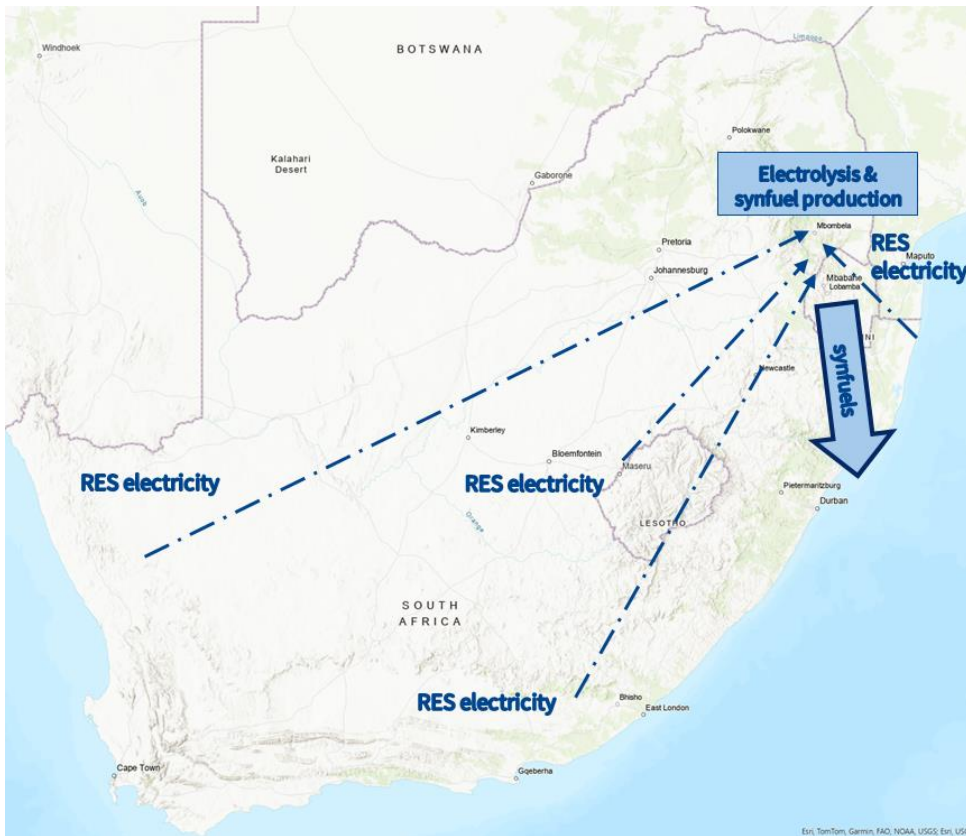
Figure 34 Renewable electricity is transported to Sasol’s facilities through transmission grid, where synfuels are produced and transported to the Port of Durban (own elaboration based on google maps)
