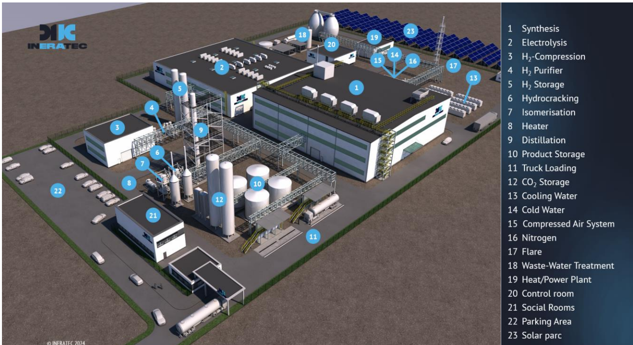
Figure 12. 3D Visualisation of 50.000 t/a e-Fuel plant.
