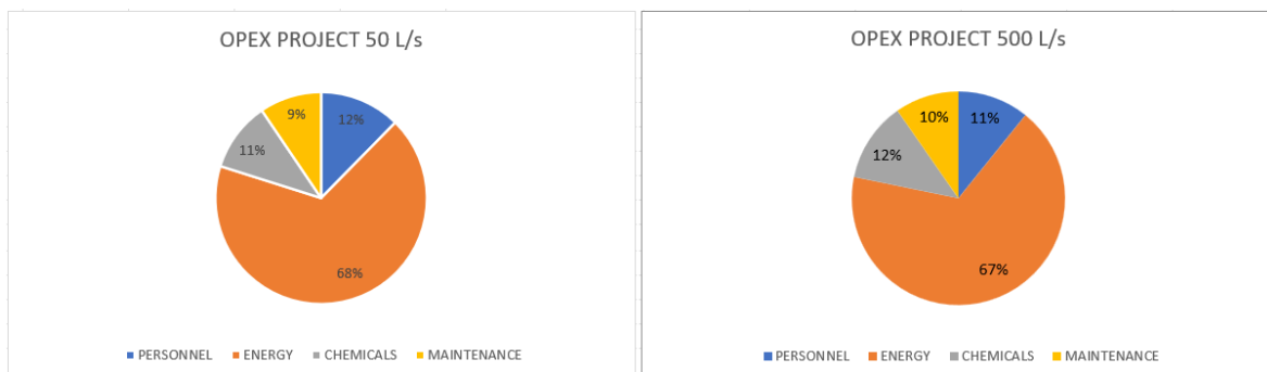
Figure 2: Distribution of operational costs for a 50 l/s plant and a 500 l/s plant. Source: (Self-generated, 2023).
