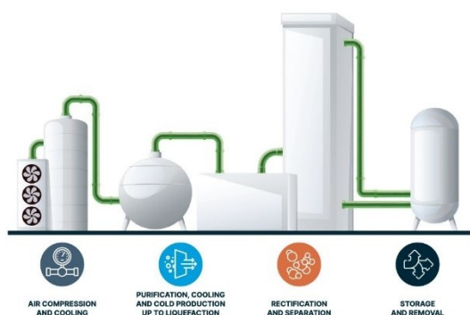
Figure 3: Process stages involved in air separation (HEROSE, 2024)
