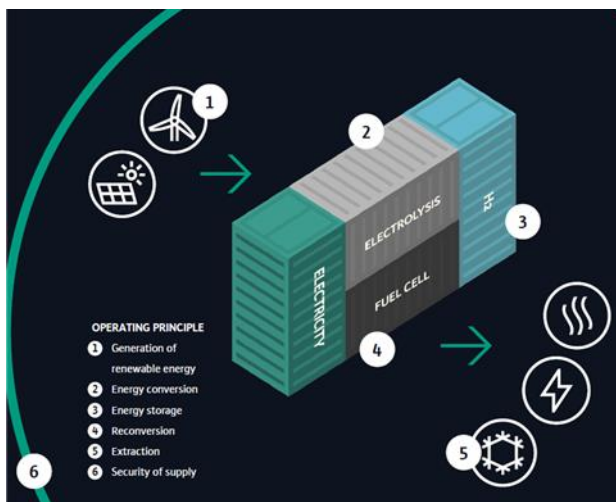
Fig. 2: Modular and intelligent industrial H2POWERPLANT concept scheme from Wilo. Published by WILO SE.
