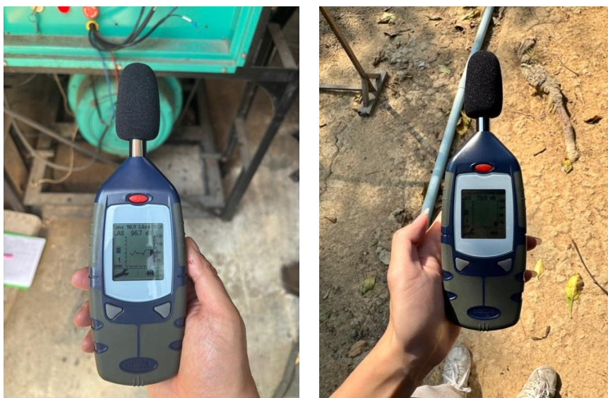
Figure 13 Sound emission in the technical building (left: 96.7 dB) and outside (right: 90.3 dB) the staff buildings (Source: EGS-plan (Bangkok) Co., Ltd.)
