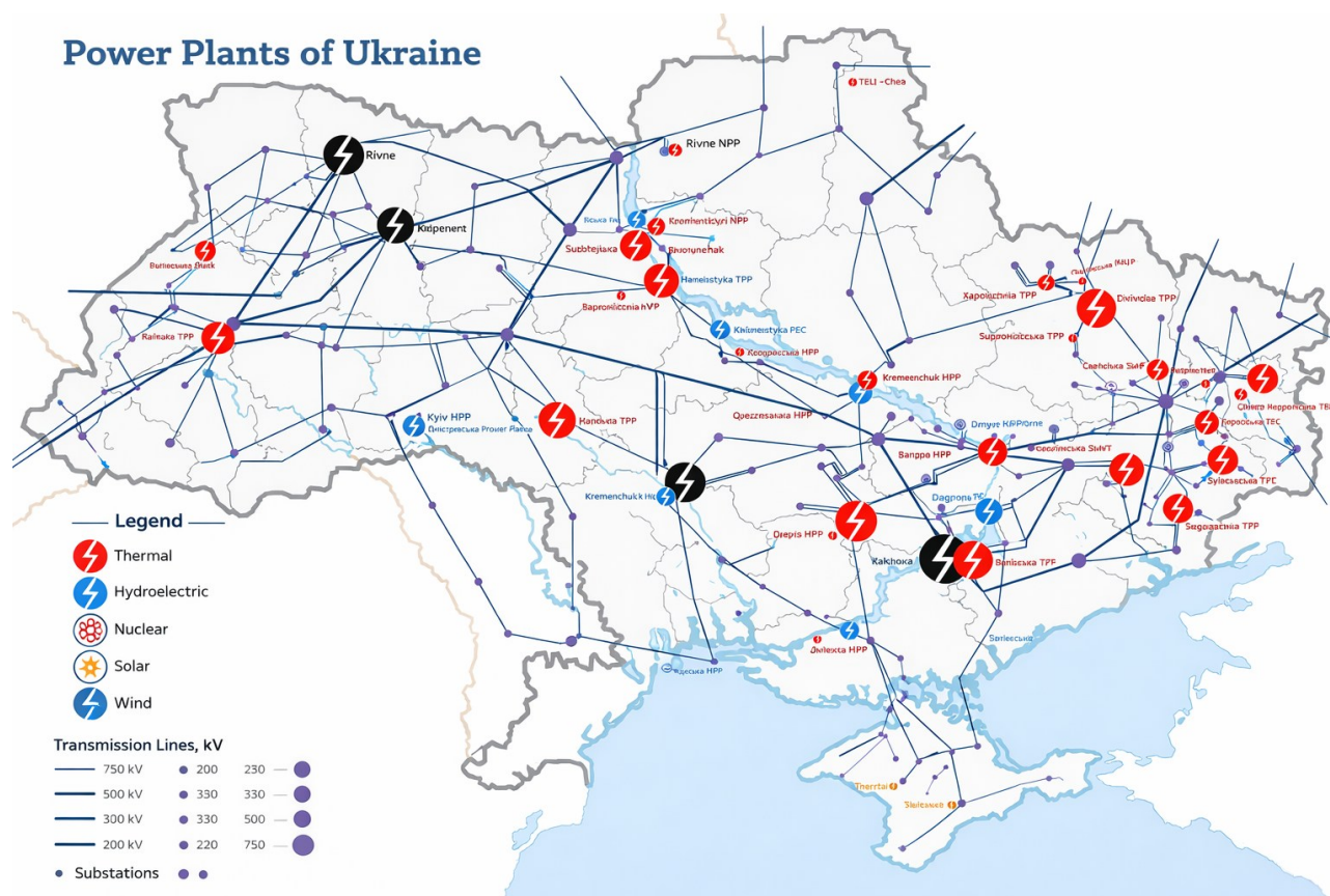
Figure 2-2: Electricity generation and transmission map of Ukraine, showing power plant types and high-voltage lines [161]
